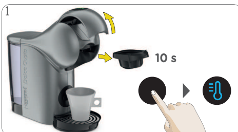
Open the locking handle. The machine switches on automatically. Touch the temperature selection icon within 10 seconds after starting the machine to change to cold mode (blue). A cold beverage can be prepared immediately.
